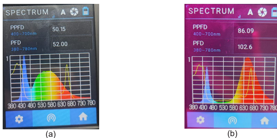
Figure 3. Wavelength measurement of the light spectrum of (a) white LED, (b) purple LED using a light meter
